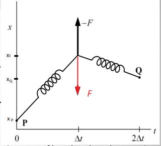
Segment of length x plotted versus time. Tension modelled as fixed ends P, Q with fictitious springs of identical  $k = m/(\Delta t)^2$
